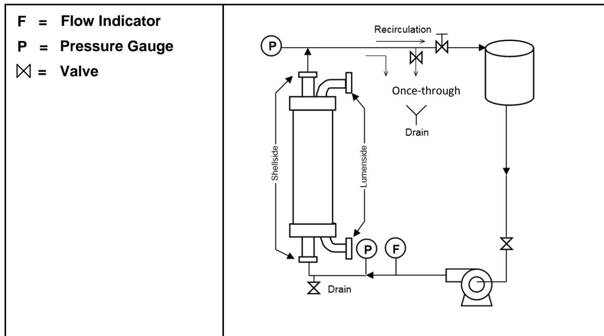
Illustration 2: Flow Schematic for Severe Biological Soil Removal
